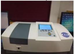
Figure 1 : Double beam UV Visible spectrophotometer
