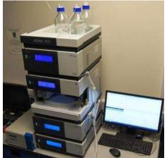
Figure 3: HPLC- High performance liquid chromatography
